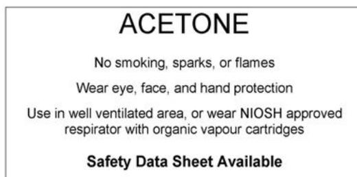
**Figure 2. Example of workplace label**
