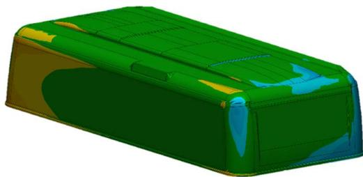
**Figure 5:** Deviation map of model vs. scan. Green areas indicate deviation of less than 6.35mm (1/4"), within tolerance
