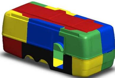
**Figure 4:** The trailer was segmented into 17 parts for Phase I.
