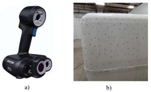
Figure 2: a) GoScan 3D scanner from CREAFORM, b) trailer segment ready for scanning, marked with positioning targets to maximize accuracy
